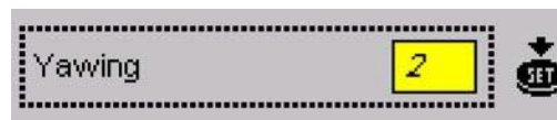
Figure 56: Example of a request to press SET after a parameter has been changed
