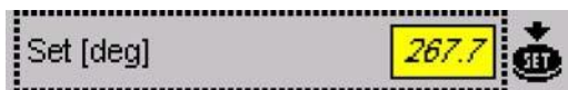
Figure 41: Example of a request to press SET after a parameter has been changed
