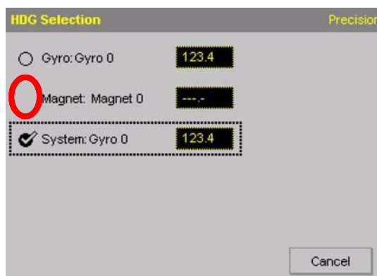
Figure 47: Heading source selection ("Page" function) - heading source not available or INS
