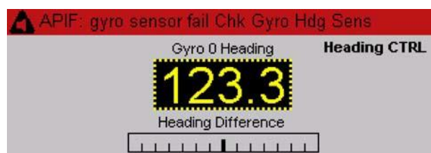
Figure 68: Alert messages at the NautoPilot® Operator Unit (example for short text)
