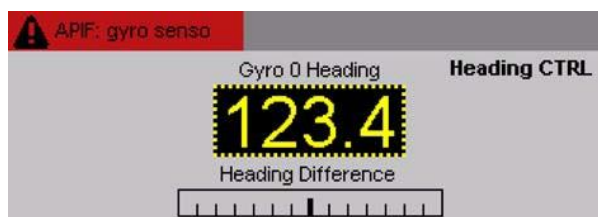
Figure 68: Alert messages at the NautoPilot® Operator Unit (example for short text)
