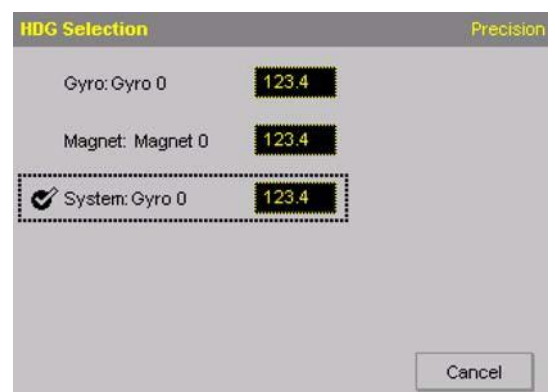
Figure 47: Heading source selection ("Page" function) - heading source not available or INS
